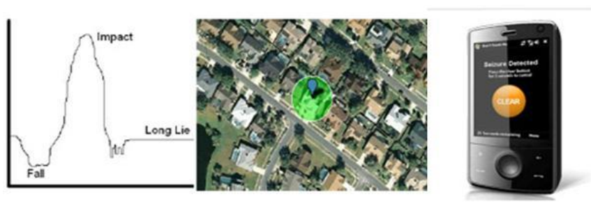
Figure 3: The detection of a fall and its location using ifall together with an Epdetect alert
